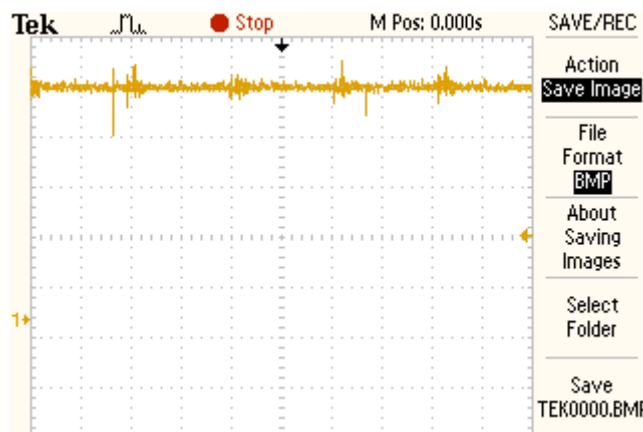
Fig.11.Output of MQ 135 gas sensor for 3gm of liquid ammonia
