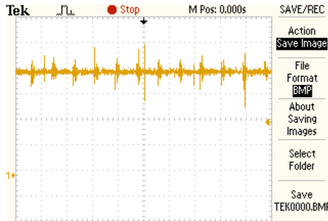
Fig.9.Output of MQ 135 gas sensor for 1gm of liquid ammonia
