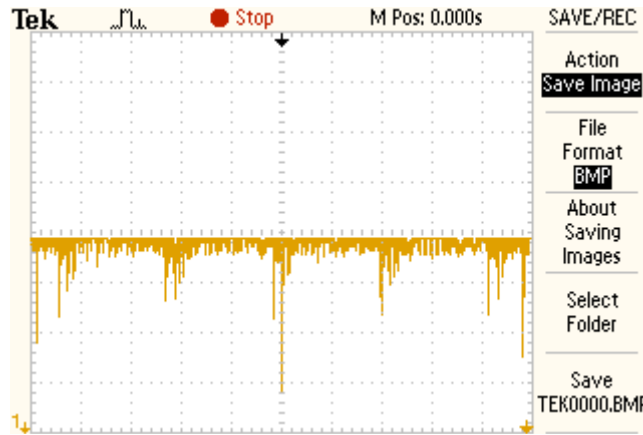
Fig.5.Output of TGS 826 gas sensor for 1gm of liquid ammonia
