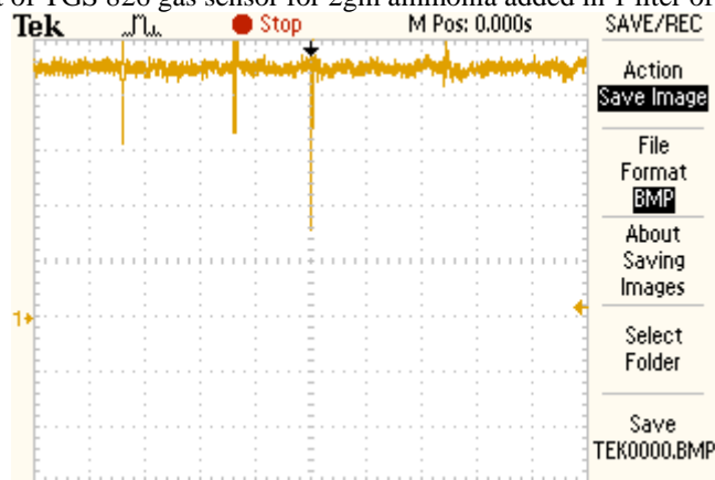
Fig.11. Output of TGS 826 gas sensor for 3gm ammonia added in 1 liter of distilled water
