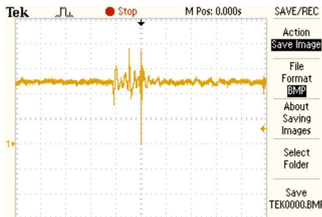
Fig.6. Output of TGS 826 gas sensor for 2gm of liquid ammonia
