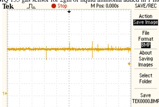
Fig.14. Output of MQ 135 gas sensor for 3gm of liquid ammonia added in 1 liter of distilled water
