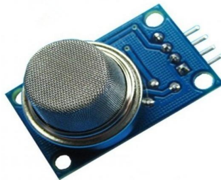
Fig. 3. Ammonia gas sensor fixed on base
